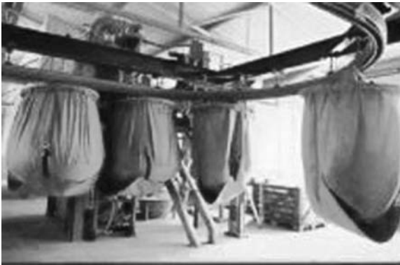
18.26 Flexible bulk containers [65].
