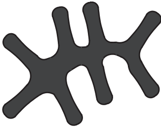
7.4 '4DG' fiber cross-section with deep grooves.
